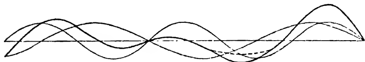
Fig. 61. The response of the ear-drum to two simple tones sounded simultaneously. As in fig. 60, a part of the thick curve is replaced by that shown by the broken line.
